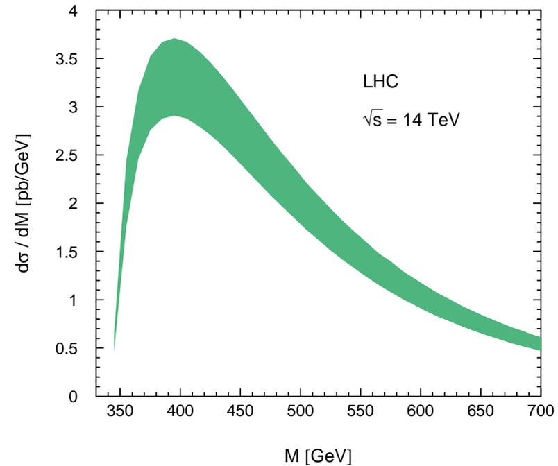
**Left:** Invariant mass distribution  $d\sigma/dM$  from NRQCD and for a fixed NLO for LHC with  $\sqrt{s} = 14$  TeV. The bands are due to scale variation for  $\mathcal{L} \otimes F$  from  $m_t$  to  $4m_t$ .
