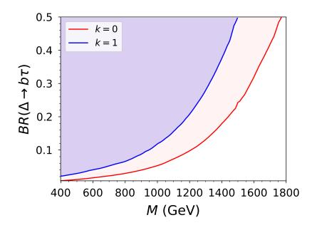
Figure 5: Reinterpretation from [110]. The main assumptions are  $BR(\Delta \to b\tau) = BR(\Delta \to t\nu)$ and that the opened second generation decay is invisible to the analysis, and hence only affects the fiducial cross-section  $\sigma(pp \to \Delta\Delta^*) \times (BR_{\Delta}^{3rd})^2$
