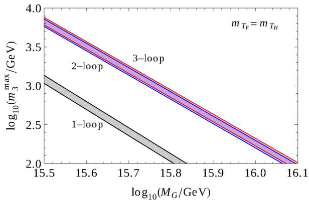
FIG. 6: The maximal value of the effective triplet mass  $m_3$  as a function of the unification scale  $M_G$ . The black, blue and red bands (from bottom-left to top-right) correspond respectively to the one-, two- and three-loop running analysis. The three-loop result is obtained by taking  $m_{T_F} = m_{T_H}$ . The error bands are due to the  $1\sigma$  uncertainties on the low-energy couplings  $\alpha_1(M_Z)$  and  $\alpha_2(M_Z)$  (cf. Eqs. (26)–(27)).
