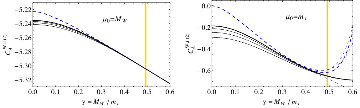
**Figure 2:**  $C_A^{W,(2)}$  as a function of  $y = M_W/m_t$  for the charm (left) and top quark sector (right). The (blue) dashed lines are obtained in the limit  $y \ll 1$ , and the (grey) solid line for  $y \approx 1$ . Thinner lines contain less terms in the expansions. The physical region for  $y$  is indicated by the (yellow) vertical band.
